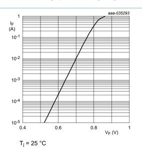
Fig. 2. Forward current as a function of forward voltage; typical values (HPZR-C5V6)
