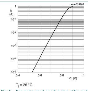
Fig. 5. Forward current as a function of forward voltage; typical values (HPZR-C68)
