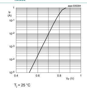
Fig. 3. Forward current as a function of forward voltage; typical values (HPZR-C7V0)
