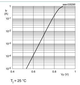
Fig. 4. Forward current as a function of forward voltage; typical values (HPZR-C8V2)
