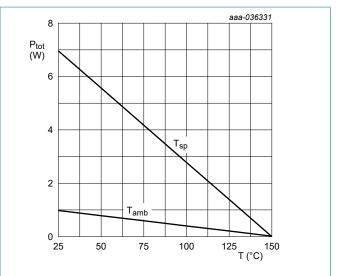
Fig. 6. Total power dissipation as a function of temperature; maximum values
